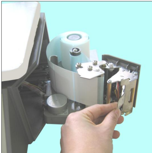
① Open the thermal printer head
